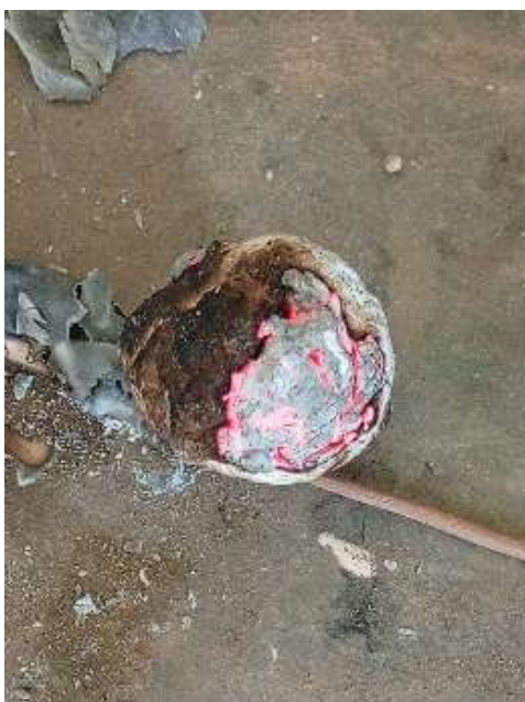
Figure 3. Paper Charcoal ( T_2 ) heat duration and it's ignition and combustion time.
